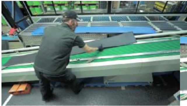
First the operator places the tread in between the slides
